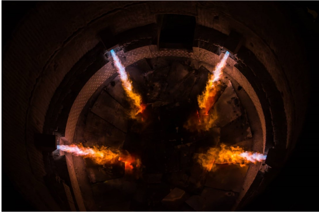
Figure 4.9: [42] Oxygen and gas burners (Primetals - EAF RCB Injection Technology) in operation [42].
